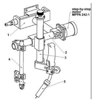
Figure 3. Positioning device for the welding head
